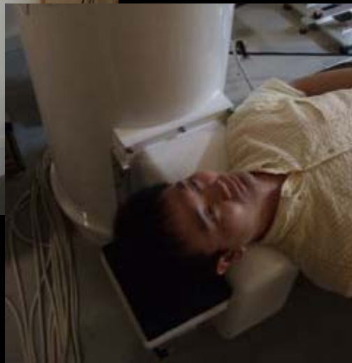
Biomagnetometer for SCEF measurements
