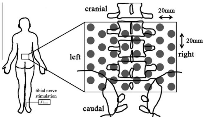
**Fig. 2.** CEAFs were recorded at 35 or 40 points over the skin surface after stimulation of the tibial nerve. Measurement points were arranged in a  $5 \times 7$  or  $5 \times 8$  matrix, and the distance between each point was 20 mm in both the longitudinal and lateral directions.
