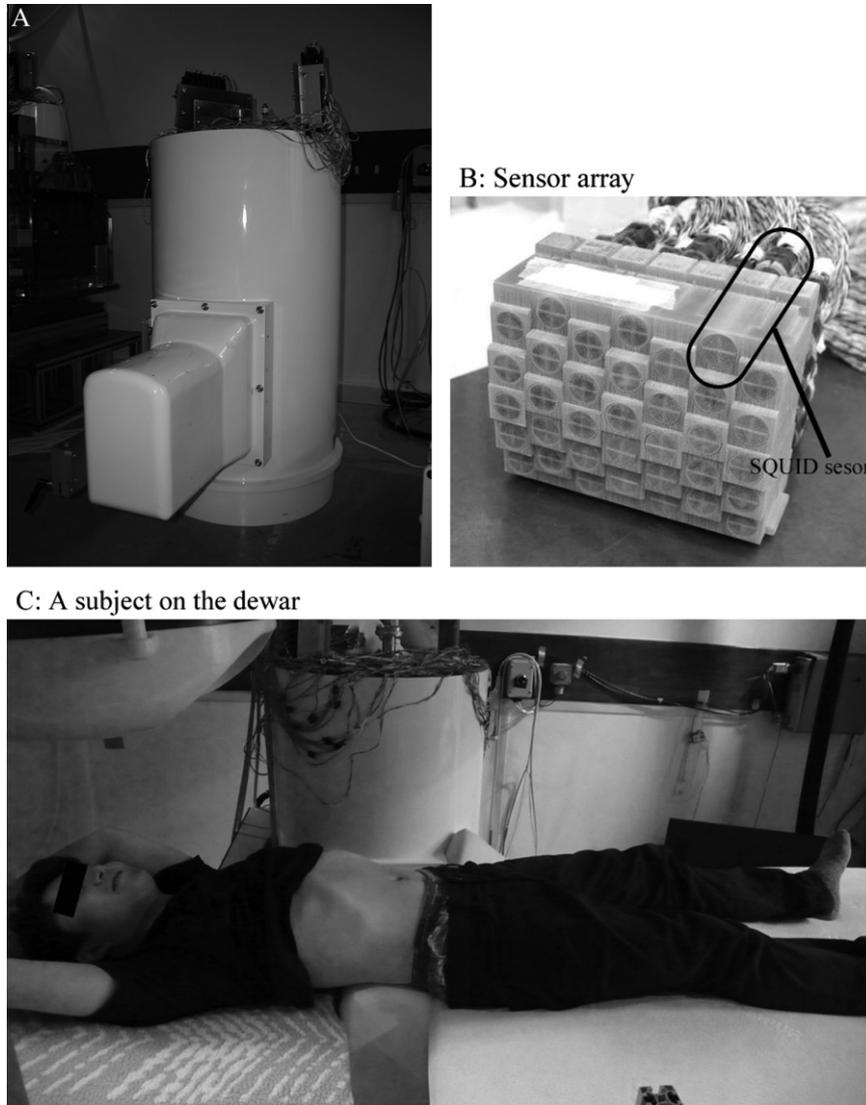
**Fig. 1.** (A) Vertical, cylinder-shaped cryostat with a sensor area protruding from the side. (B) An array of SQUID vector gradiometers with a  $5 \times 8$  matrix-like arrangement. (C) The sensor surface is curved to fit to the lordosis of the subject's lumbar spine.
